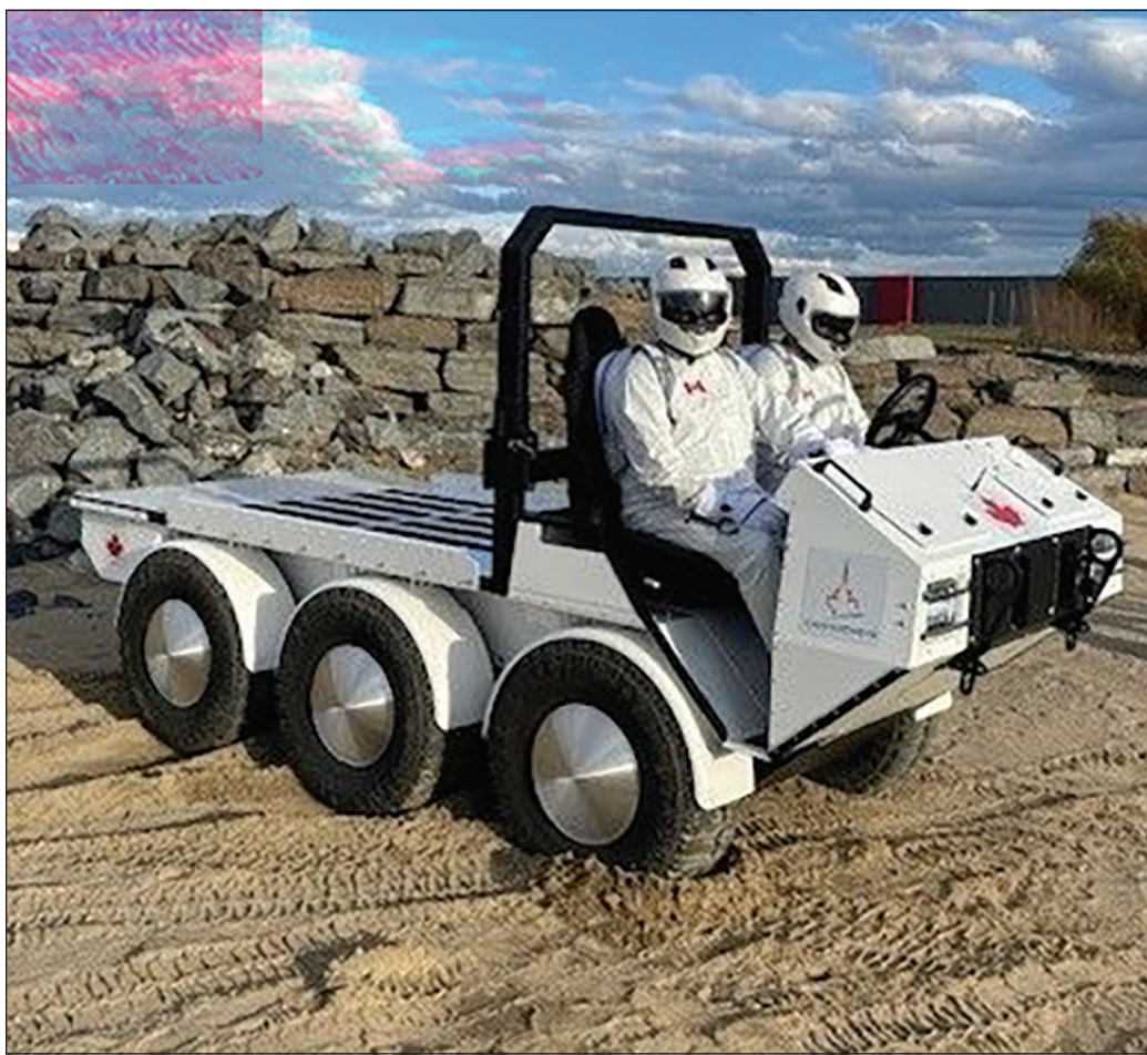
A large Canadensys lunar test vehicle is being used to develop operational concepts for lunar missions. Sample LUV configurations are being evaluated by Canadensys.
