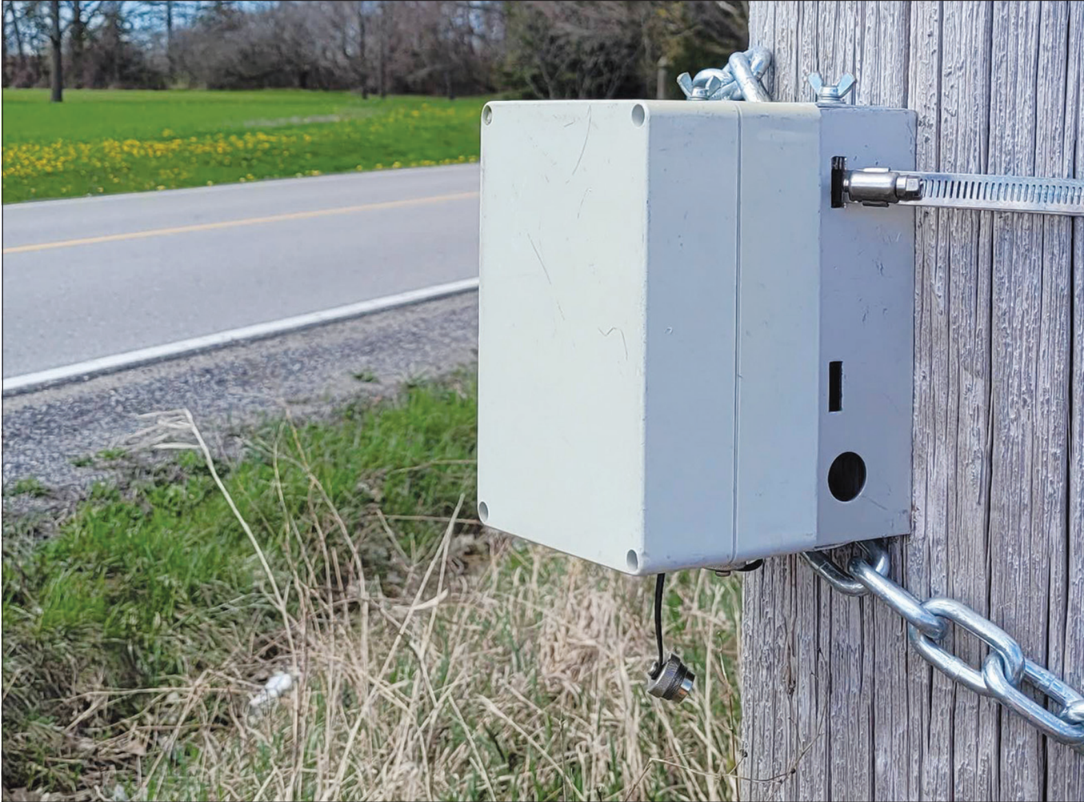
The Armadillo Tracker is the newest tool in King Township's arsenal. It will be used to check data, as part of King's traffic calming measures.
