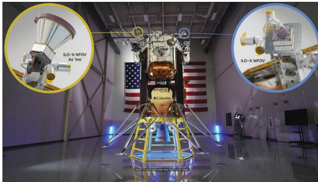
The Canadensys Near Field of View (NFOV) and Wide Field of View (WFOV) optical instruments designed and built for the ILO-X mission are mounted on top of the IM-1 Lunar Lander, arrived at the NASA Kennedy Space Center and is being prepared for launch.
